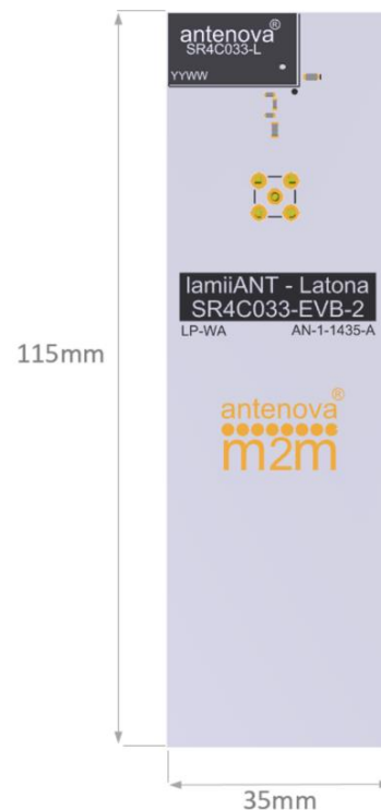
SR4C033-EVB-2 Evaluation Board (For SR4C033-L)
