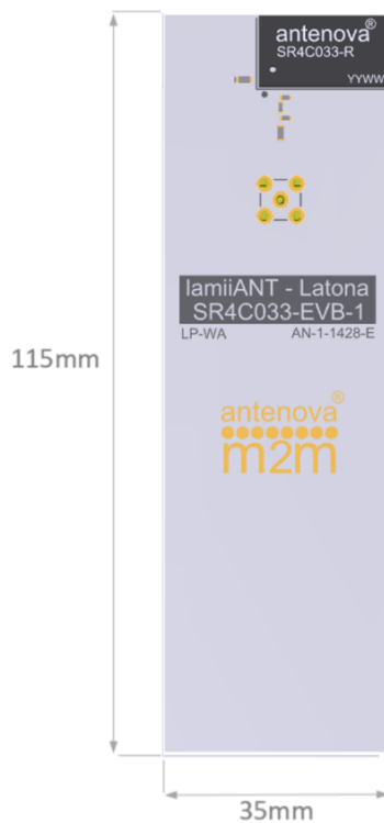
SR4C033-EVB-1 Evaluation Board (For SR4C033-R)
