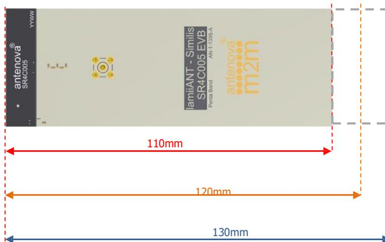
**Passive Efficiency vs. PCB length**
