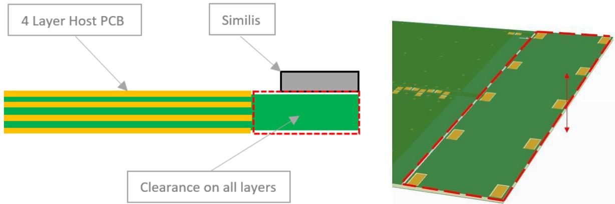
Placement of components and GND with traces adjacent to the antenna should maintain a minimum clearance of 15mm from either side. The antenna should be therefore placed in the corner to only have one side effected.
