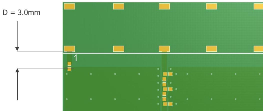
The distance  $D$  is the gap required from the antenna SMD pad edge to the ground plane. This should be maintained along the edge the antenna is placed.
